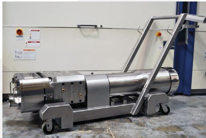
UNIBLOC PD-652 with custom front cover discharge and cart
