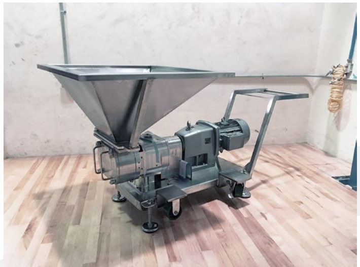
UNIBLOC PD-550 with custom hopper and cart
